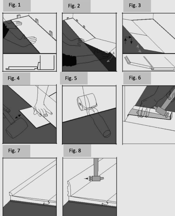
Once the floor is fitted, remove the spacers; sweep the floor with a soft brush. Fix the skirting boards or suitable edge trim to cover the expansion gaps. These should be fixed to the wall and not the floor (Fig. 7 & 8).
