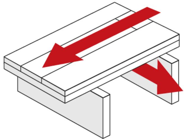
Check with the joist or truss Manufacturer to determine if cross-bracing is allowed with that system. Should it not be compatible with the joist or truss Manufacturer, sheathing the sub floor with a second layer of CD or better grade plywood would then be the only option. (See double layer sub floors section).
